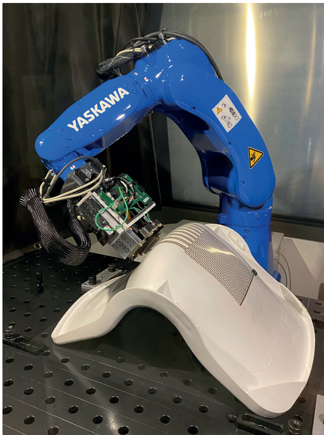
Robot-guided inkjet printing of a heating conductor structure for a heatable seat shell: test stand at Fraunhofer ENAS with Yaskawa GP8 robot. (Photo © Fraunhofer ENAS)
