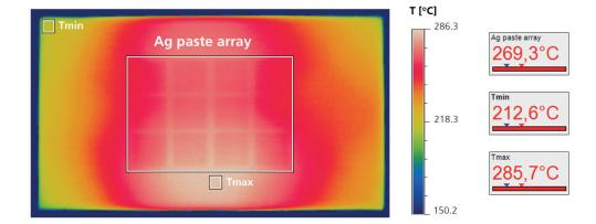
IR image of inductive heating of the multi-chip setup with Ag paste array onto the DBC substrate. The target temperature of 300 °C is reached in only five seconds. (Image © Fraunhofer ENAS)
