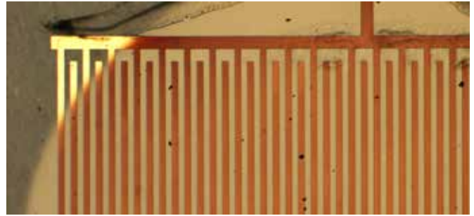
Metal electrodes on a flexible Parylene substrate, coated with a gas sensitive layer for the realization of a flexible gas sensor.
