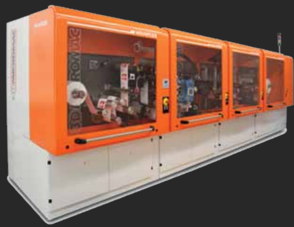
Fig. 1: First configuration of the modular R2R Digital Fabrication system microFLEX, consisting of a rotary screen printing and a drop-on-demand inkjet module. The system is a joint development of 3D-Micromac AG and Fraunhofer ENAS under the supervision of Tino Petsch and Prof. Reinhard R. Baumann ( http://www.3d-micromac.com/press-release/articles/processing-of-thin-film-materials.html ).
