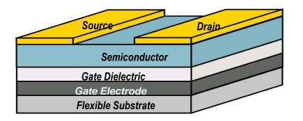
Schematic structure of a back-gated thin-film transistor (TFT) on a flexible substrate
