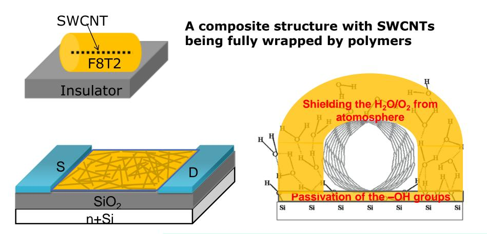
Source of hysteresis for TFTs with  $SiO_2$  as dielectric: (1)  $SiO_2$  surface bounded water ( $\equiv SiOH$  groups) (2)  $H_2O/O_2$  in the ambient atomosphere
