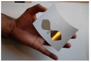
Quadrate Bowtie Antenna for UHF RFID Band
