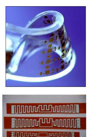
Robust UHF Antennas with low ink consumption and high gain
